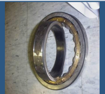
Picture of actual bearing that was replaced. One can see obvious spalling of the inner ring proving it was near failure
