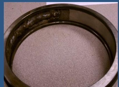
Outer race bearing defect of gear A bearing found through vibration analysis
