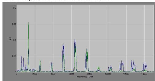
**Enveloped Gs is a very important tool in early detection of bearing problems. I have also found it to be an excellent tool in determining which bearing is bad on a two bearing pulley.** Low frequency travels very well through the shaft from bearing to bearing, however high frequency does not travel as well.
